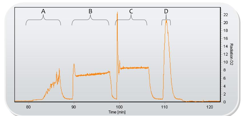
Image 4: Radioactive elution profile from hydroximate resin column. A. Loading dissolved foil (in 2mL 6M HCl + 5mL H<sub>2</sub>O) onto resin, B. Washing resin with 10mL 2M HCl, C. Washing resin with 10mL H<sub>2</sub>O, D. Elution of <sup>89</sup>Zr with 1.0M oxalic acid in 1.0-1.2mL final volume.
