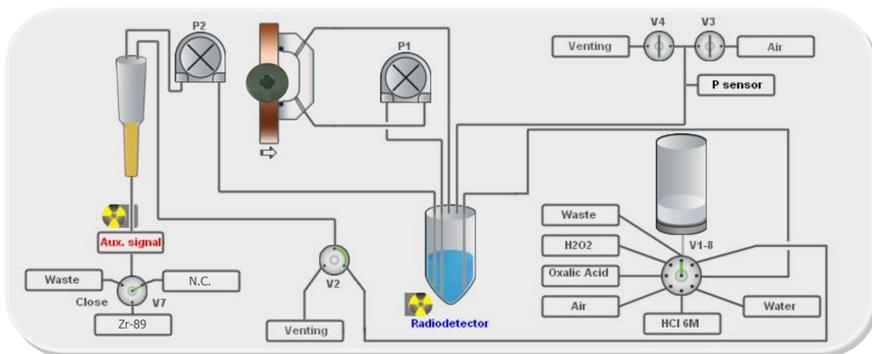
Image 2: Schematic of IBA Pinctada Metal dissolution/purification module setup for <sup>89</sup>Zr production.
