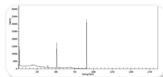
Image 5: Spectrum of  $\gamma$ -ray emissions from a purified <sup>89</sup>Zr sample 2hrs after EOB
