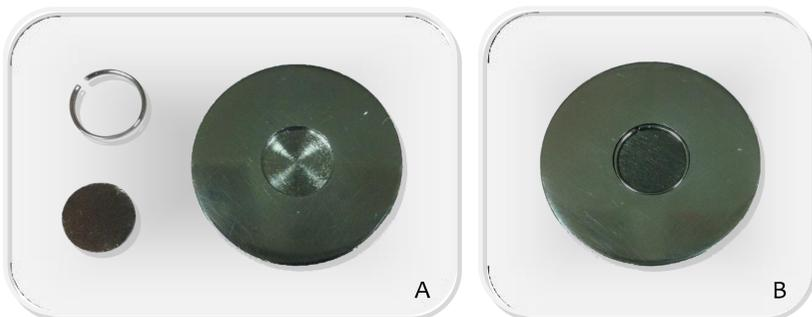
Image 1: (A) Disassembled Pt target foil cradle, Y-foil and Pt containment ring. (B) Assembled target ready for irradiation.
