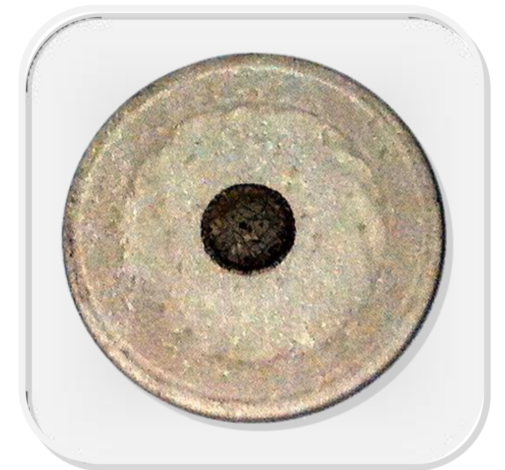
Image 3: Ag disk (24mm \varnothing ) with 47.4 \mu m thick (13.0mg, 6mm \varnothing ) 64 Ni plating
