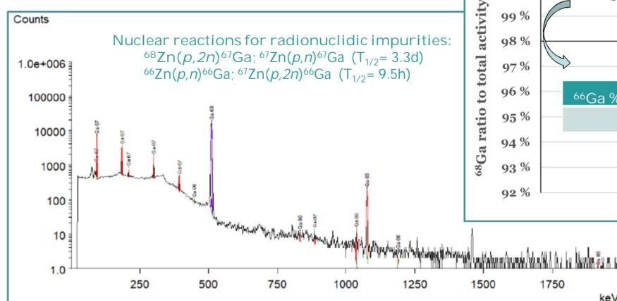
Fig. 5. Gamma-spectrum of the purified  $^{68}\text{Ga}$ -target solution at 8.5 h from EOB. The production conditions were 1 hour irradiation on 94 mg of  $^{68}\text{Zn}$  using 40  $\mu\text{A}$  beam current and approximately 14 MeV beam energy (two Nb-foils).
