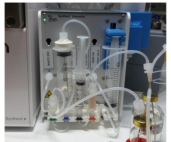
Fig. 4. IBA Synthera® Extension module equipped with Fluidomica purification kit for  $^{68}\text{Ga}$ -target solution
