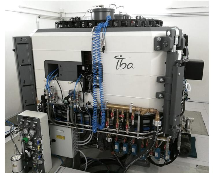
Fig. 2. IBA Cyclone® KIUBE 180 cyclotron at the HUS Medical Imaging Center
