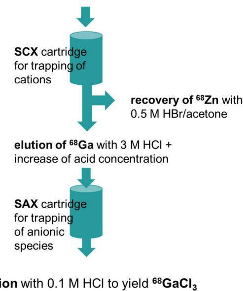
Fig. 3. Separation scheme for  $^{68}\text{Ga}$  in  $^{68}\text{Zn}(\text{NO}_3)_2$  solution. The overall time for the procedure is 35 min.
