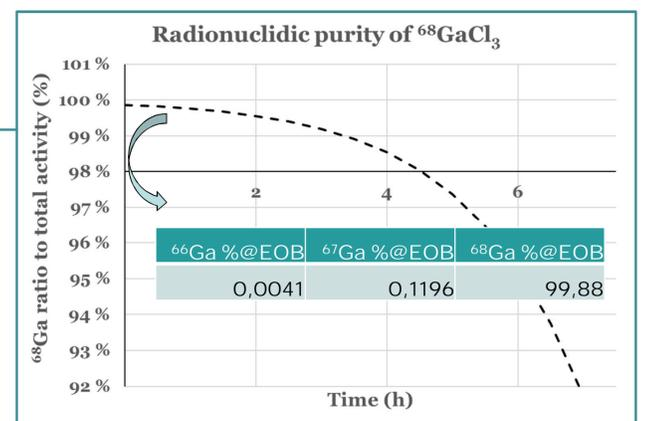
Fig. 6. Radionuclidic purity of  $^{68}\text{GaCl}_3$  at various time-points. Results are calculated from the HPGe measurements that were continued until 27h from EOB.
