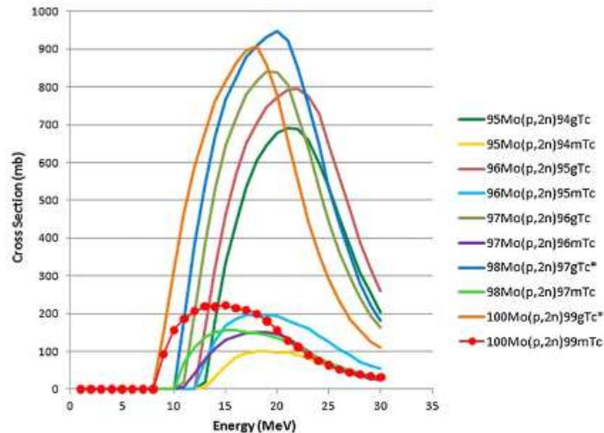
**Figure 4.** Comparison of the  $^{100}\text{Mo}(p,2n)^{99\text{m}}\text{Tc}$  excitation function to the other radioactive and stable technetium isotopes (isomeric and ground states) which are produced through the (p,2n) reaction. The excitation function for  $^{99\text{m}}\text{Tc}$  is marked with red circles and stable isotopes are marked by an asterisk.
