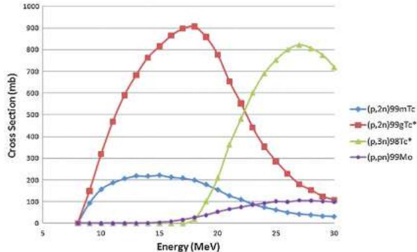
**Figure 2.** Excitation functions corresponding to the  $^{100}\text{Mo}+p$  reaction products with the highest cross sections in the investigated energy range. Stable isotopes are marked by an asterisk.
