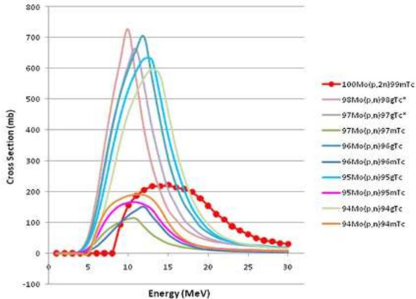
**Figure 3.** Comparison of the  $^{100}\text{Mo}(p,2n)^{99\text{m}}\text{Tc}$  excitation function to the six other technetium isotopes (isomeric and ground states) which are produced through the (p,n) reaction. The excitation function for  $^{99\text{m}}\text{Tc}$  is marked with red circles and stable isotopes are marked by an asterisk.
