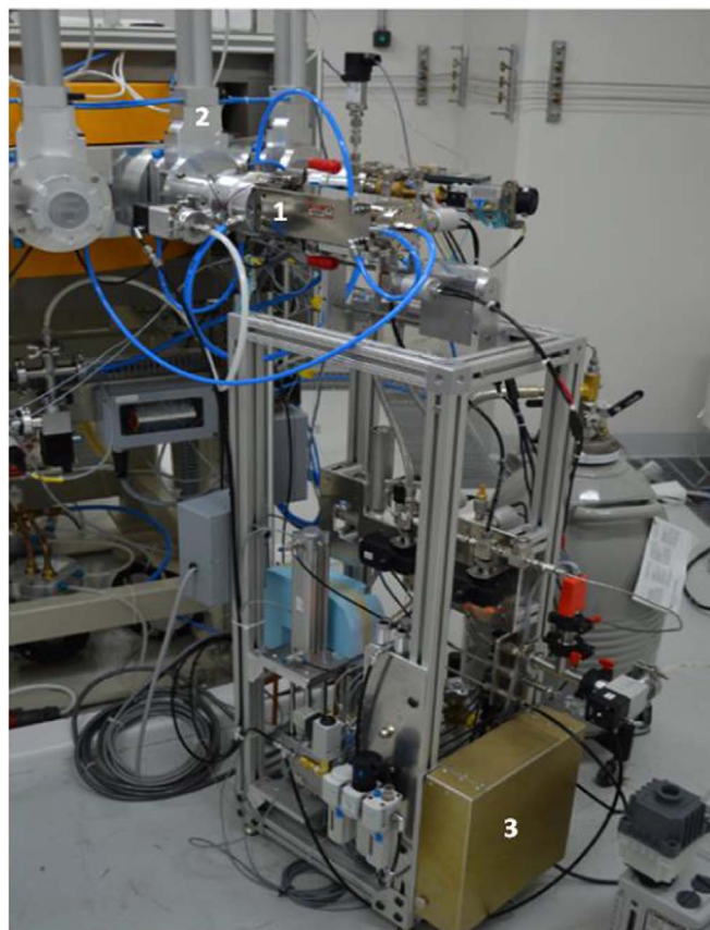
Fig. 4. Krypton target attached to the cyclotron beamline. Description of the target component is as follow: 1) target body, 2) cyclotron beam valve and 3) current reading circuitry.
